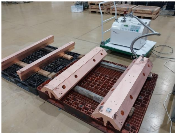
Fig. 4. Vacuum leak check after plug brazing.
