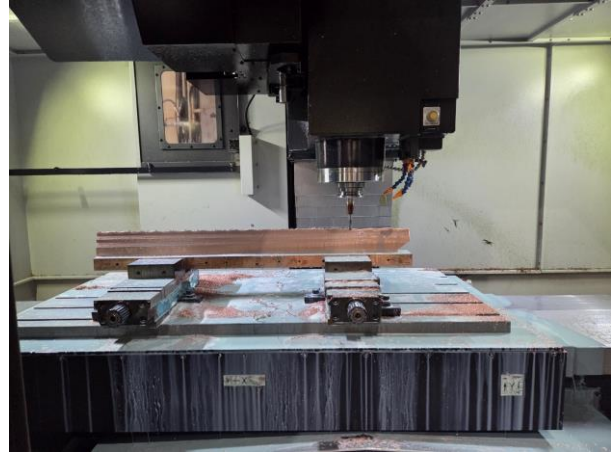
Fig. 5. RFQ minor vane under final machining.
