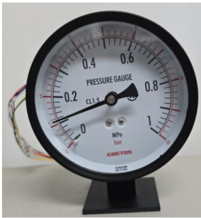
Fig. 3. Example image of the fabricated gauge with motor attachment.
