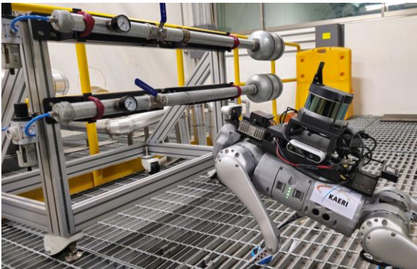
Fig. 1. Example of analog gauges on pipelines and a quadruped robot for automatic reading in a nuclear facility.
