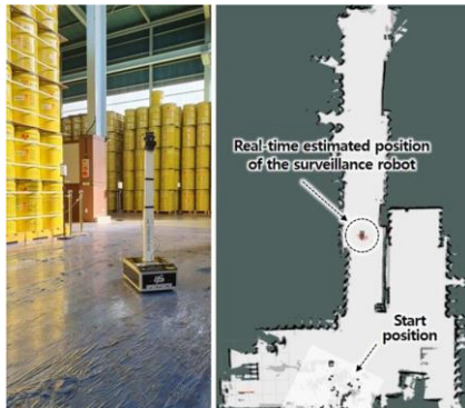
Fig. 1. The surveillance robot and the generated map data in the real radioactive waste storage facility. (Reprinted from [Lee et al., 2021])
