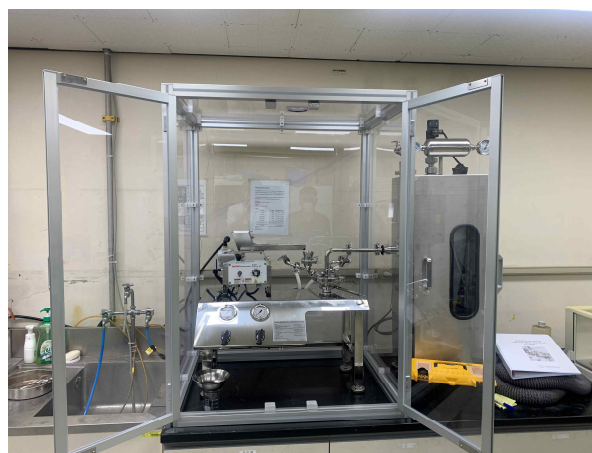
Figure 1. 2-inch jet-milling equipment
