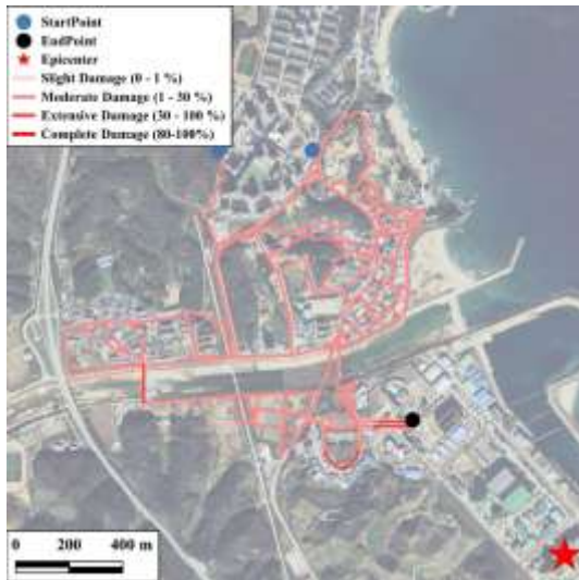
Fig. 2. Road network damage assessment results for Mw 7 (approx. PGA 0.5g)
