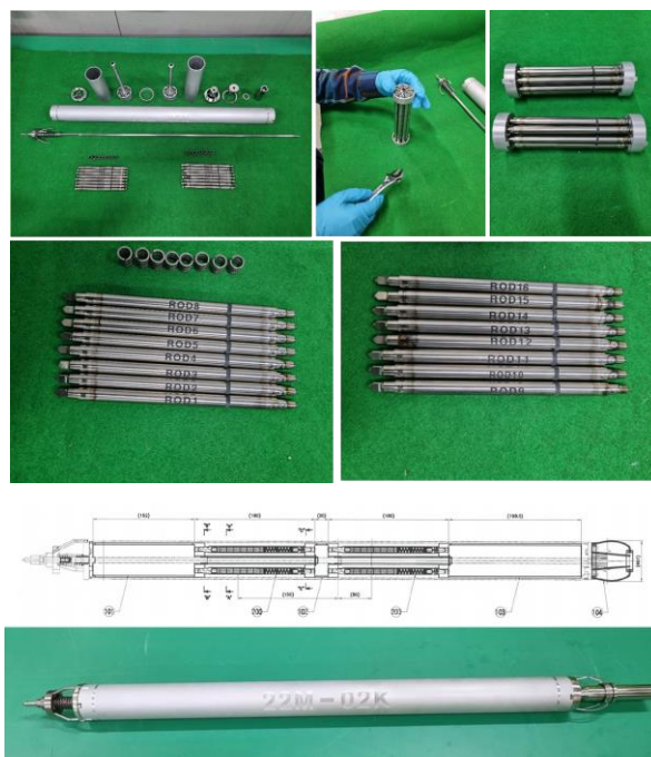
Fig. 1. Test rods, capsule design and assembled test capsule.
