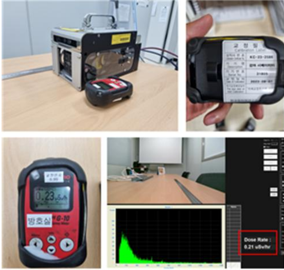
Fig. 3. Performance evaluation results for dose rate estimation.
