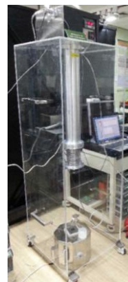
Fig. 2. Dynamic bubbler system for density measurement.
