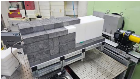
Fig. 4. Experimental setup for evaluating neutron shielding efficiency of the concrete sample
