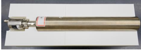
Fig. 2. ^3\text{He} proportional counter tube used as neutron detector with holder
