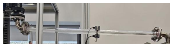
Fig. 6. Horizontal stratified-flow during the drainage
