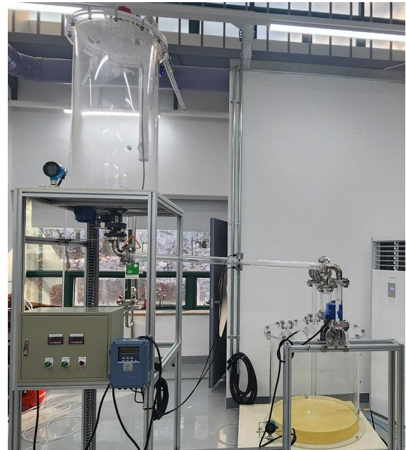
Fig. 1. K-MSR drain system scaled experimental apparatus
