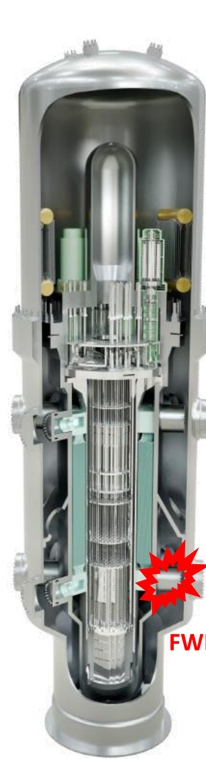
Figure 1. i-SMR FWLB Location
