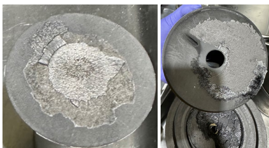
Fig. 3. Atomization Component Parts after first experiment (C2405 batch) : Disk(Left), Carbon Parts(Right)
