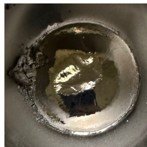
Fig. 7. U_3Si_2 alloy ingot in the ceramic crucible after fourth experiment (C2408 batch)
