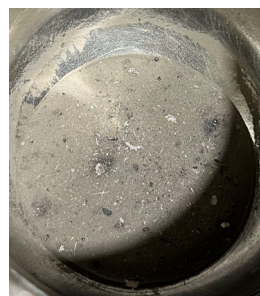
Fig. 6. U_3Si_2 powder of C2407 batch before sieving
