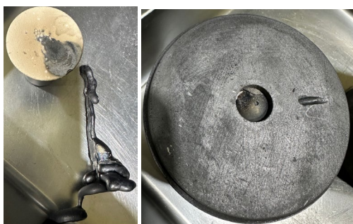
Fig. 4. Atomization Component Parts after second experiment (C2406 batch) : Disk and Ingot(Left), Carbon Parts(Right)
