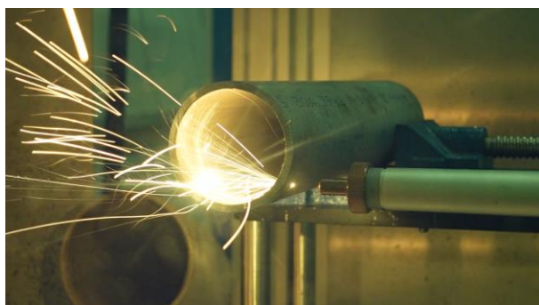
Fig. 2. Laser cutting of the stainless steel pipe in progress.
