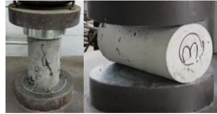
Fig. 6. Concrete test method (Left : compression, Right : Tensile)
