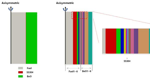
Fig. 2. Single-region (left) and six-region (right) spatial homogenization.
