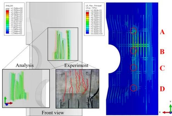
Figure 2 : XFEM-based crack growth analysis in concrete (left) and maximum principal strain distribution in liner (right)
