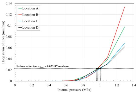
Figure 3 : Hoop strain of liner according to internal pressure
