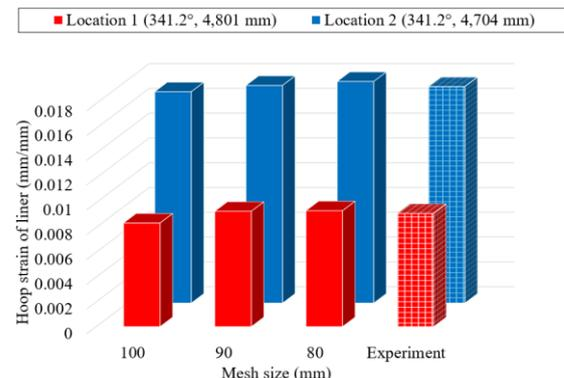
Figure 1 : Comparison of mesh sensitivity analysis results with experimental data at 3.3 P<sub>d</sub>
