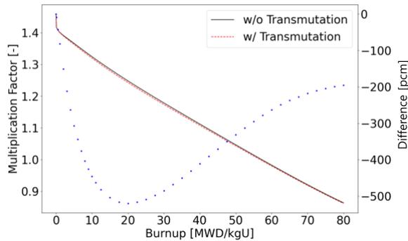
Fig. 3. Multiplication factor of BeO reflector against burnup
