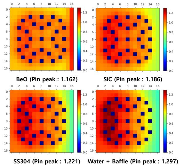
Fig. 5 Pin power distribution of reactor neighboring FA
