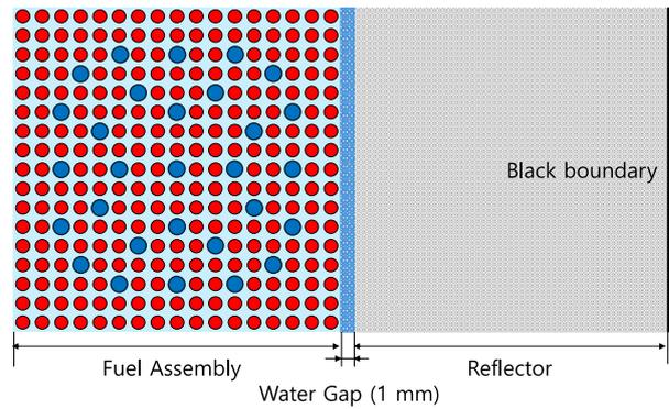
Fig. 1 Reflector model neighboring LEU+ fuel assembly
