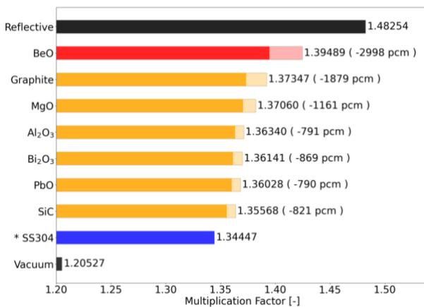
Fig. 4 Multiplication factor of non-metallic reflectors w/ SS304 coating
