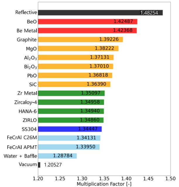
Fig. 2 Multiplication factor of reflectors
