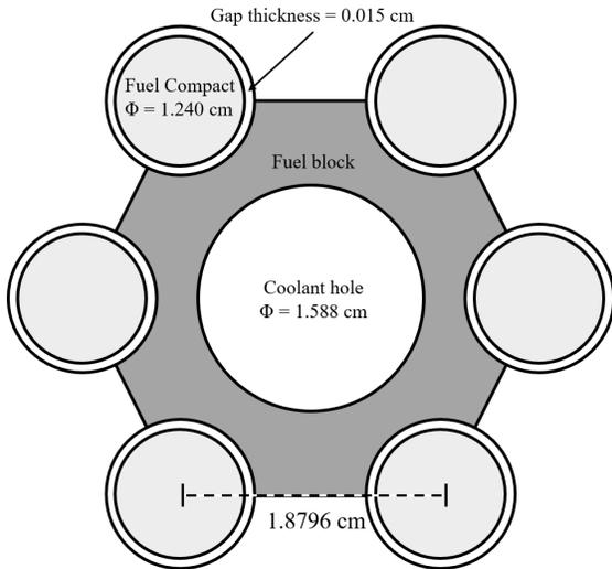
Figure 1. Unit cell of graphite block.
