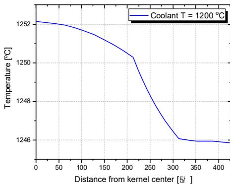
Figure 9. Temperature gradient of TRISO-coated fuel particles at the center of the fuel compact at a coolant temperature of 1200°C.
