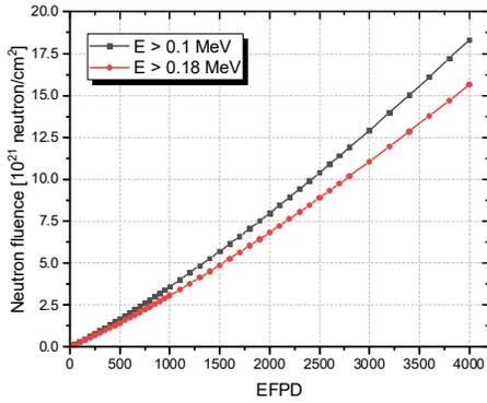
Figure 4. Fast neutron fluence variation with EFPD.
