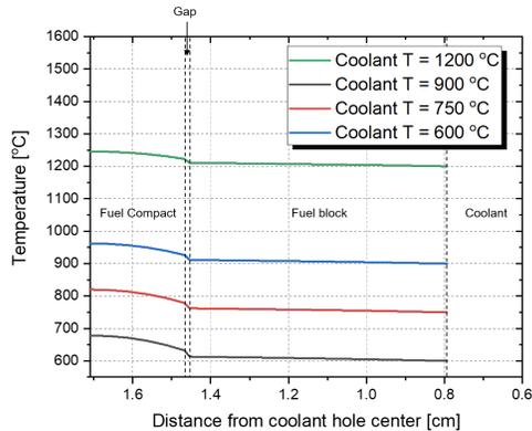
Figure 5. Temperature distribution variation with coolant temperature.
