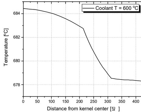
Figure 6. Temperature gradient of TRISO-coated fuel particles at the center of the fuel compact at a coolant temperature of 600°C.
