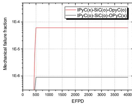
Figure 12. Mechanical failure fraction under a coolant temperature of 1200 °C.
