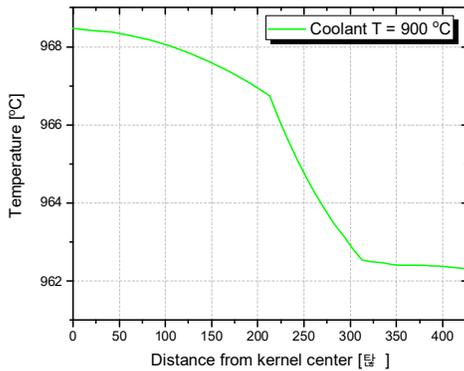
Figure 8. Temperature gradient of TRISO-coated fuel particles at the center of the fuel compact at a coolant temperature of 900°C.
