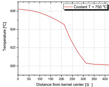
Figure 7. Temperature gradient of TRISO-coated fuel particles at the center of the fuel compact at a coolant temperature of 750°C.
