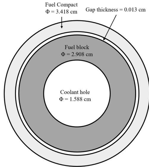
Figure 2. Transformation of the unit cell into an equivalent cylindrical model
