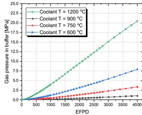
Figure 10. Total gas pressure variation inside TRISO-coated fuel particles.
