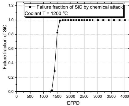
Figure 11. Failure fraction of SiC due to chemical attack under a coolant temperature of 1200 °C.
