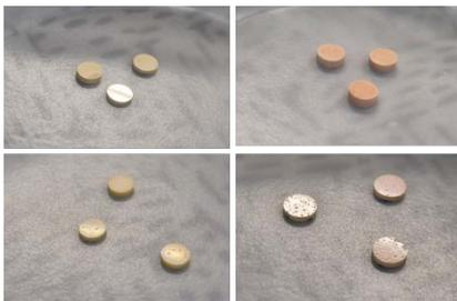
Fig 1. Fabricated Undoped/Doped Gadolinia Samples
