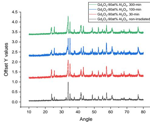
Fig 4. t-to-2t XRD pattern of Irradiated Gd<sub>2</sub>O<sub>3</sub>-90at% Al<sub>2</sub>O<sub>3</sub>
