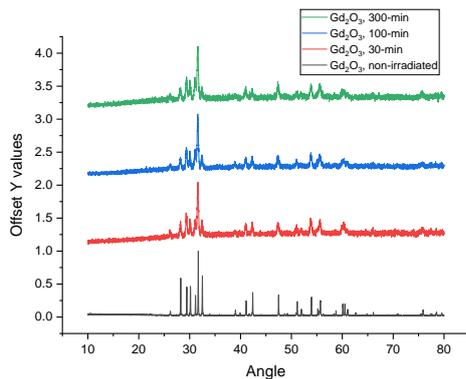
Fig 3. t-to-2t XRD pattern of Irradiated Gd<sub>2</sub>O<sub>3</sub>
