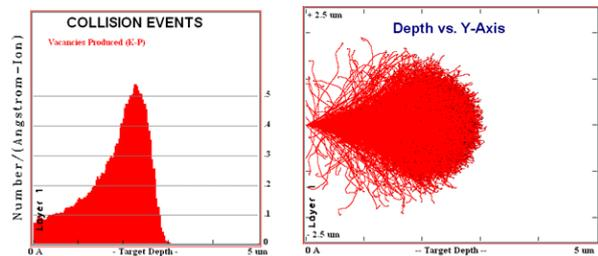
Fig 2. SRIM Simulation Result of Ar Ion Irradiated in Gadolinia. (a) Calculated dpa peaks around 2.0-2.6  $\mu m$  (b) which can be seen on the trajectory of each simulated Ar ion
