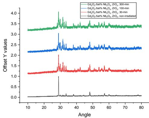
Fig 6. t-to-2t XRD pattern of Irradiated  $Gd_2O_3$ -5at%  $Nb_2O_5$ ,  $ZrO_2$
