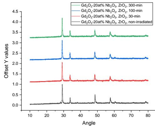
Fig 5. t-to-2t XRD pattern of Irradiated Gd<sub>2</sub>O<sub>3</sub>-20at% Nb<sub>2</sub>O<sub>5</sub>, ZrO<sub>2</sub>
