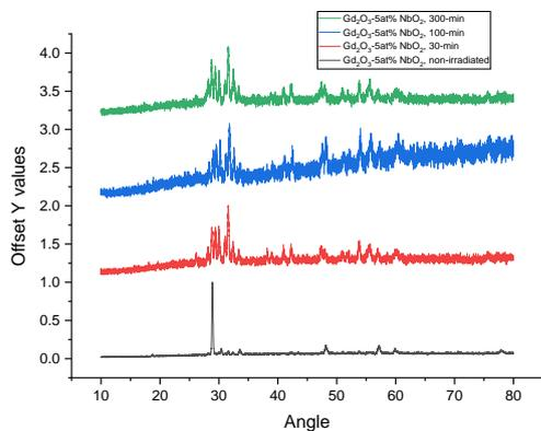
Fig 7. t-to-2t XRD pattern of Irradiated  $Gd_2O_3$ -5at%  $NbO_2$
