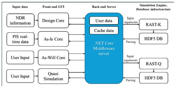
Fig. 3. The architecture of WDCT
