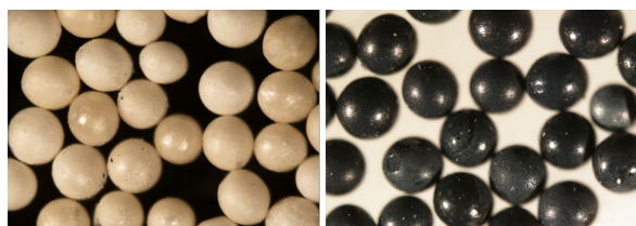
Fig. 3. Optical microscopy images of \text{ZrO}_2\text{-ZrC} surrogate fuel after heat treatment without CO (a) and with CO (b).
