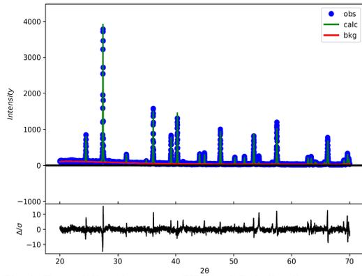
Fig. 3. X-ray diffraction pattern (XRD) of Cs-hollandites prepared via cold sinter-assisted route
