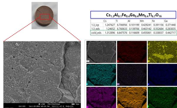
Fig. 2. Scanning electron microscopy (SEM) and images of Cs-hollandites prepared via cold sinter-assisted route
