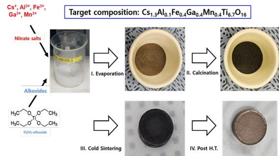
Fig. 1. Schematic diagram of hollandite fabrication process using cold-sintering route
