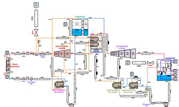
Fig. 2. MARS-KS Nodalization for i-SMR
