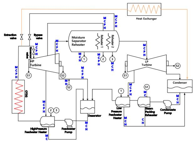
Fig. 1. Schematics of BOP for i-SMR (Basic design)
