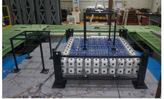
Fig. 3. Small-scale model of a metafoundation with a structure.
