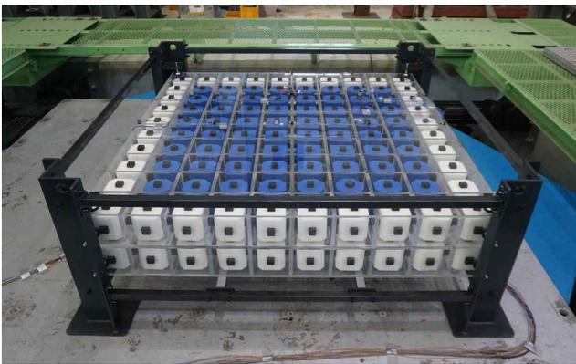
Fig. 2. Small-scale model of a metafoundation without a structure.
