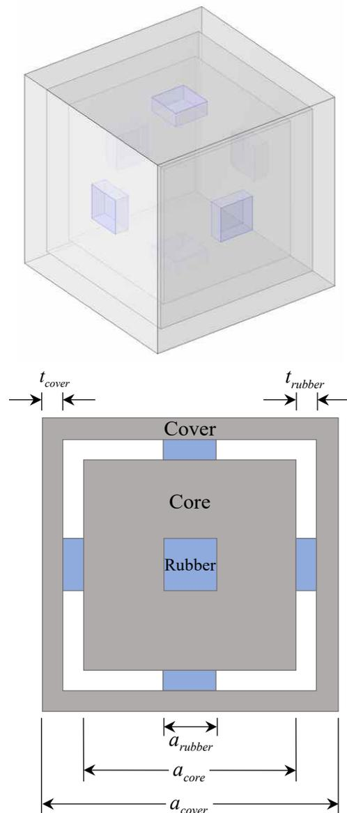
Fig. 1. Unit cell of the metafoundation.
