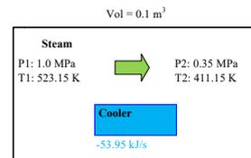
Fig. 4. Case 1: cooling process in a closed system
