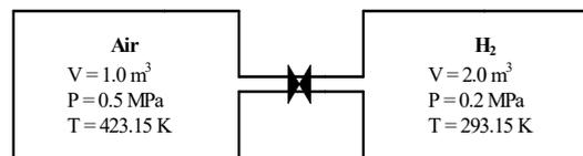
Fig. 5. Case 2: mixing of two gases
