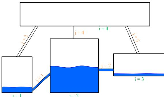
Fig. 1. Example connections between compartments and flow paths
