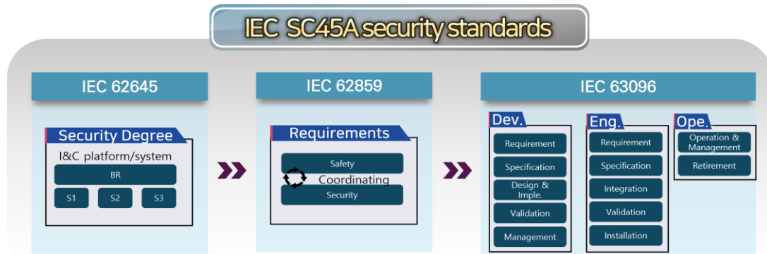
Fig. 1. Overview of IEC SC45A security standard series: IEC 62645, IEC 62859, IEC 63096
