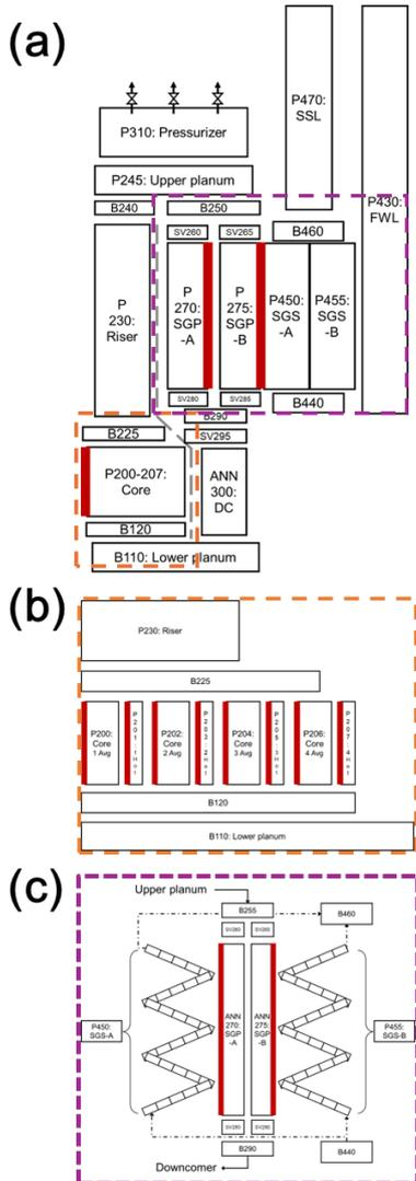
Figure 3. MARS-KS input model nodalization (a) total system, (b) core region, (c) SG region.
