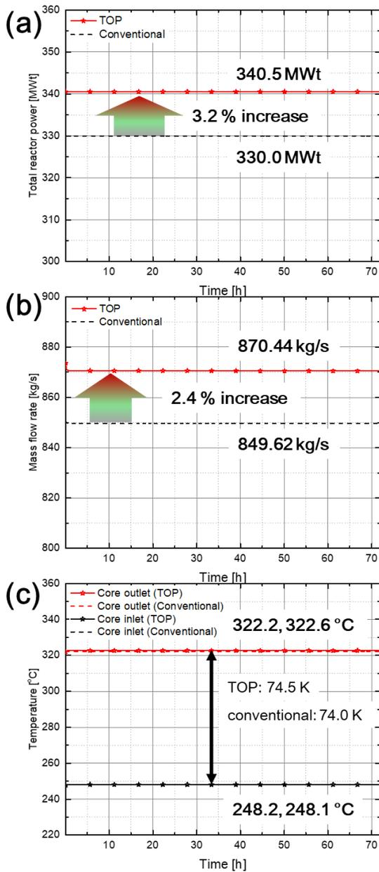
**Figure 4.** Comparison between MARS-KS results of conventional and TOP lattice core designs.
