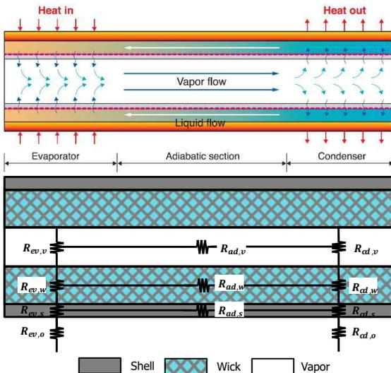
Fig. 2. Heat Pipe Heat Resistance Computer Modeling Structure
