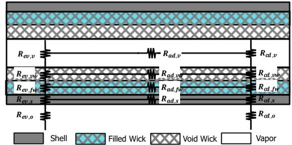
Fig. 3. Improved Heat Pipe Heat Resistance Computer Modeling Structure
