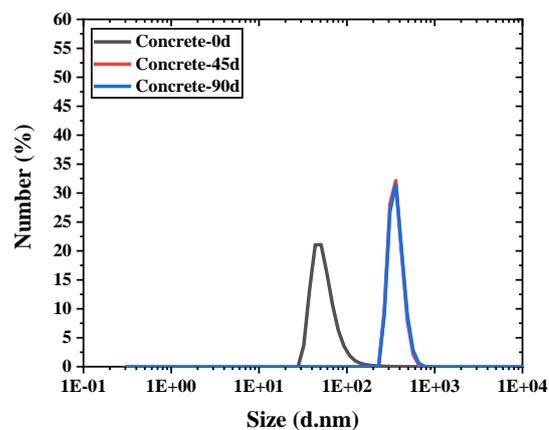
**Figure 4.** Number distribution of generated colloids in the accelerated concrete experiment
