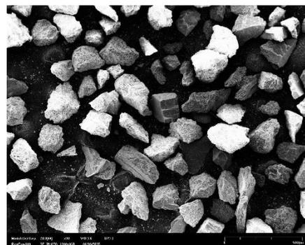
Figure 1. SEM image of crushed concrete particle
