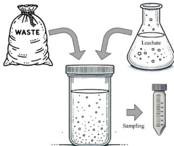
**Figure 2.** Overall experimental setup: the leachate and particulate concrete waste in a PP container for 90 days at different temperature
