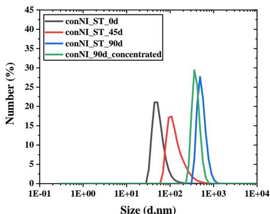
**Figure 3.** Number distribution of generated colloids in the short-term concrete experiment
