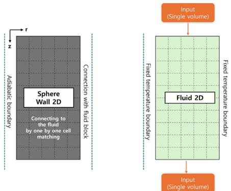
Fig 3. Nodalization of heat structure and fluid for packed bed modeling in GAMMA+
