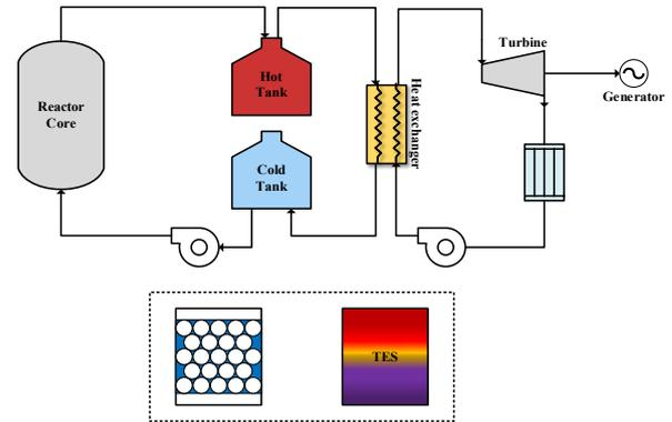
Fig 1. Overall schematic layout of TES operating diagram, two-tank (top), packed bed (left), and thermocline (right)
