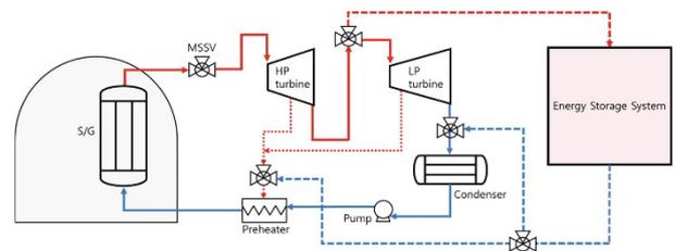
Fig 2. Conceptual diagram of integrated steam cycle of PWR power plants with energy storage system [6]
