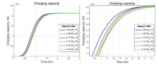
Fig 8. Charging capacity in radial direction of Packed bed at aspect ratio (left) and detail (right)
