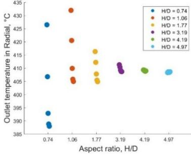
Fig 6. Temperature difference in radial direction of Packed bed for different aspect ratio
