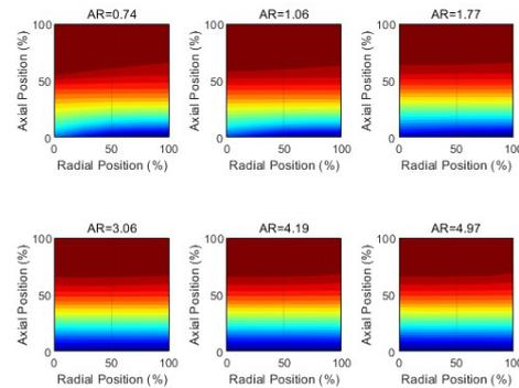
Fig 5. Temperature distribution in Packed bed for different aspect ratio at 1.5 hours charging
