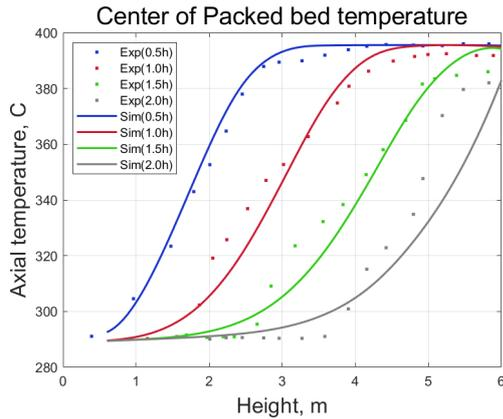
Fig 4. Validation result of Sensible heat stored in molten salt packed bed
