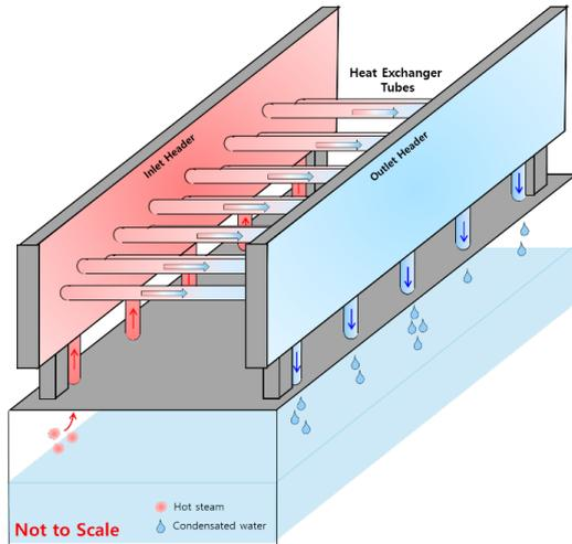
Fig. 3. Condensation heat exchanger 3D conceptual diagram
