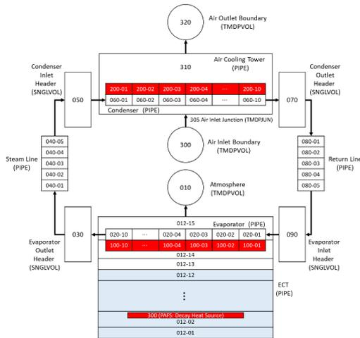
Fig. 6. LLHP Cooling Tower MARS-KS Input Geometry
