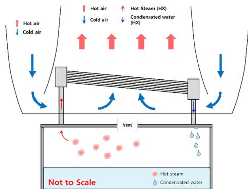
Fig. 4. Condensation heat exchanger cooling tower side view
