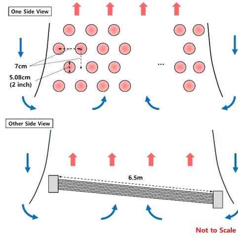
Fig. 5. Heat Exchanger Tube Design
