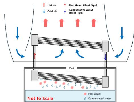
Fig. 2. Large loop heat pipe cooling tower side view
