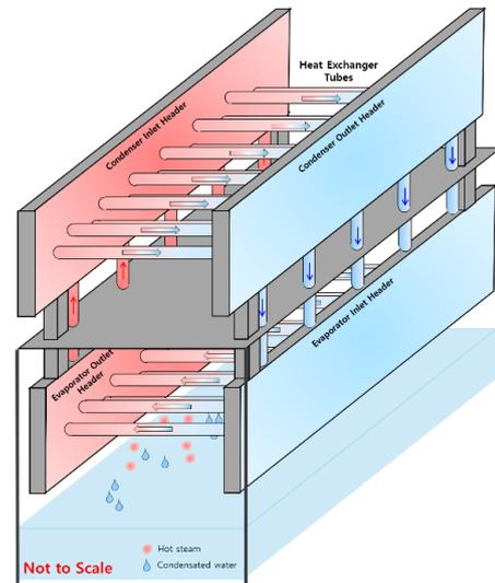
Fig. 1. Large loop heat pipe 3D conceptual diagram
