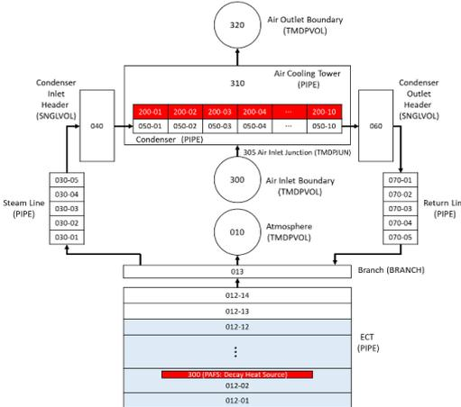
Fig. 7. CHX Cooling Tower MARS-KS Input Geometry
