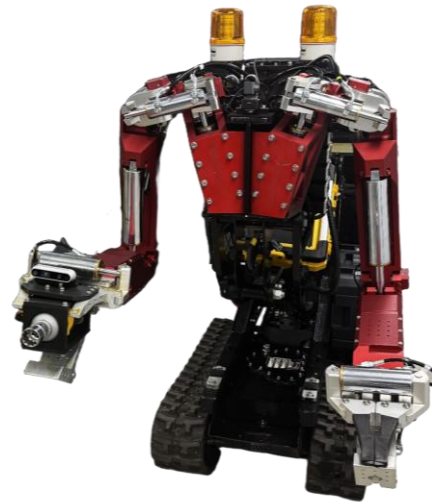
Fig. 1 ARMstrong, the hydraulic dual arm mobile manipulator
