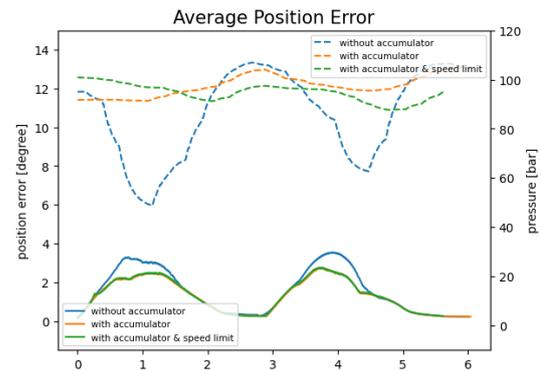
Fig. 4. Average position error of high-speed motion experiment
