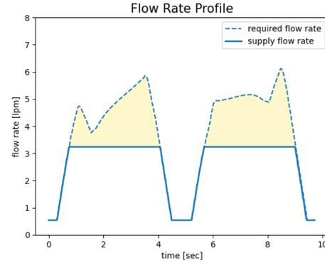
Fig. 2. Pump controller command with limited supply flow to utilize stored hydraulic fluid in the accumulator
