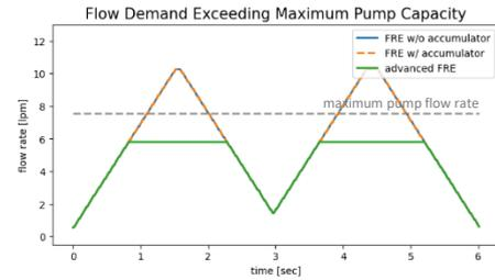
Fig. 3. Pump controller command in case of required flow rate exceeding pump capacity with FRE control without accumulator, FRE with accumulator and advanced FRC control with accumulator
