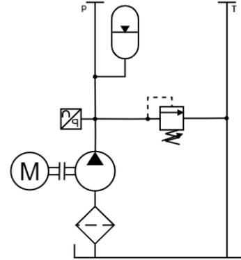
Fig. 1. Hydraulic circuit of m-HPU
