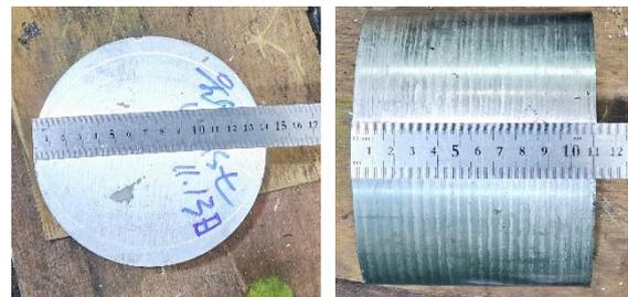
Fig. 1. High nitrogen ASS block.
