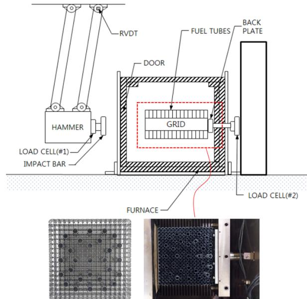
Fig. 2. Schematic of the dynamic crush test equipment
