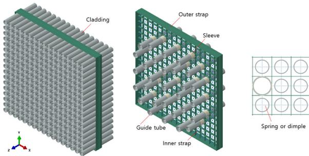
Fig. 3. Spacer grid model
