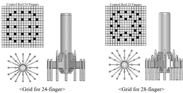
Fig. 1. Design of the spacer grid according to fingers
