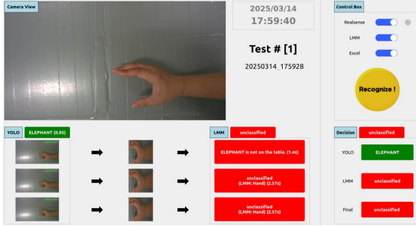
Fig. 3. Final decision: unclassified (YOLO misclassified as 'ELEPHANT', corrected by LMM)
