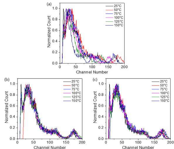
Fig. 2. Energy spectrum (a) Reference (b) Pre-compensation (c) Post-compensation
