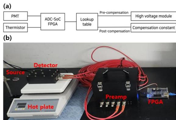
Fig. 1. (a) Schematic of temperature compensation system. (b) The preamplifier, SoC FPGA, PMT
