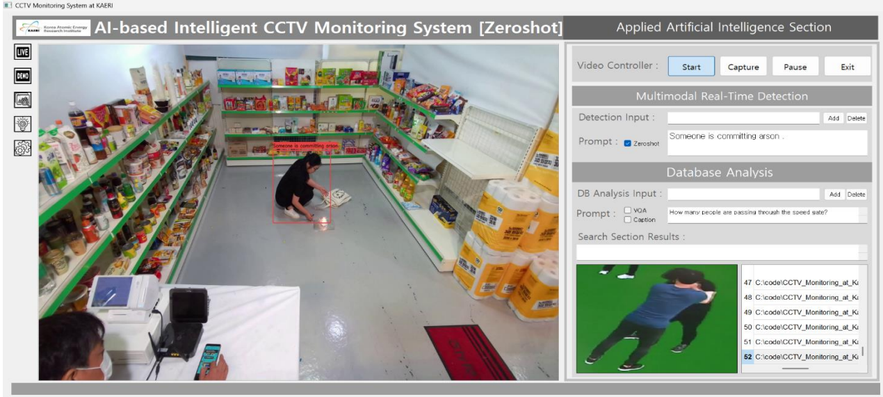
Fig. 1. This is a prototype image of an intelligent CCTV system using zero-shot learning (ZSL) to detect an individual committing arson. Due to security concerns that prohibit the use of internal images, the image displayed in the UI is sourced from the AI Hub dataset.
