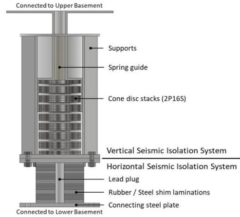
Fig. 1 Schematics of Integral 3D-LRB
