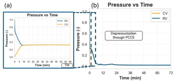
Fig 3. Pressure between RPV and CV (a) for 1 hour (b) for 72 hours analysis
