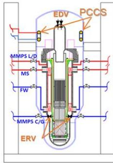
Fig 1. Diagram of i-SMR valves and pipelines
