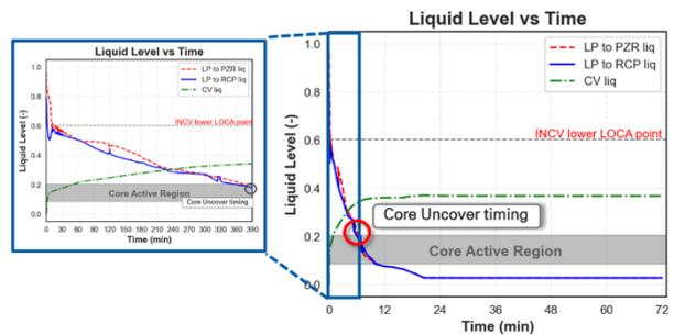
Fig 4. Water level analysis (a) from the beginning to core uncover timing (b) for the whole case scenario
