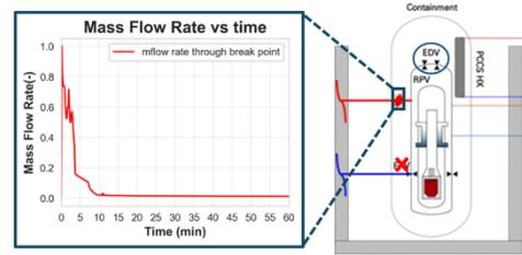
Fig 2. Diagram of i-SMR and break location with mass flow rate through break point
