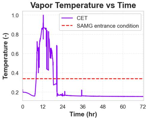
Fig 5. Core exit temperature with SAMG condition
