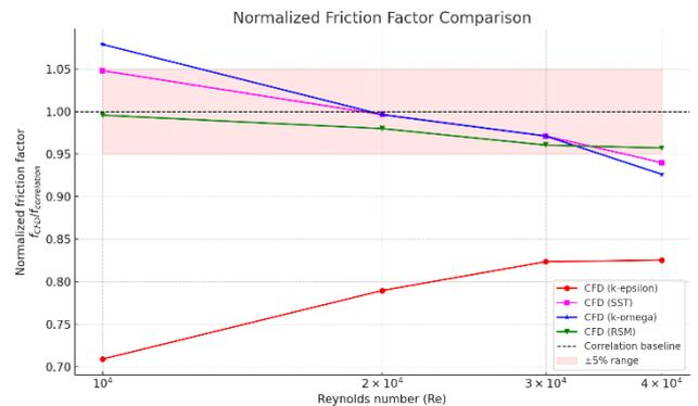
**Figure 4. Normalized friction factor ( $f_{CFD}/f_{correlation}$ ) in a helical pipe as a function of Reynolds number for different turbulence models.**
