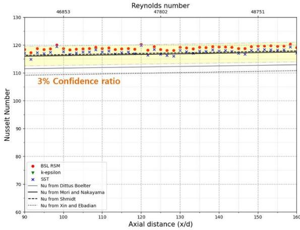
**Figure 5. Comparison of CFD-based Nusselt number with empirical correlations for different turbulence models.**
