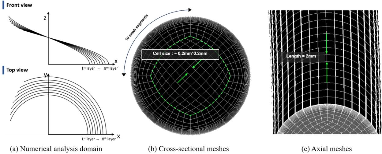
**Figure 1. CFD analysis schematic domain geometry (a) and mesh shape (View of cross-sectional mesh(b) and axial mesh(c)).**
