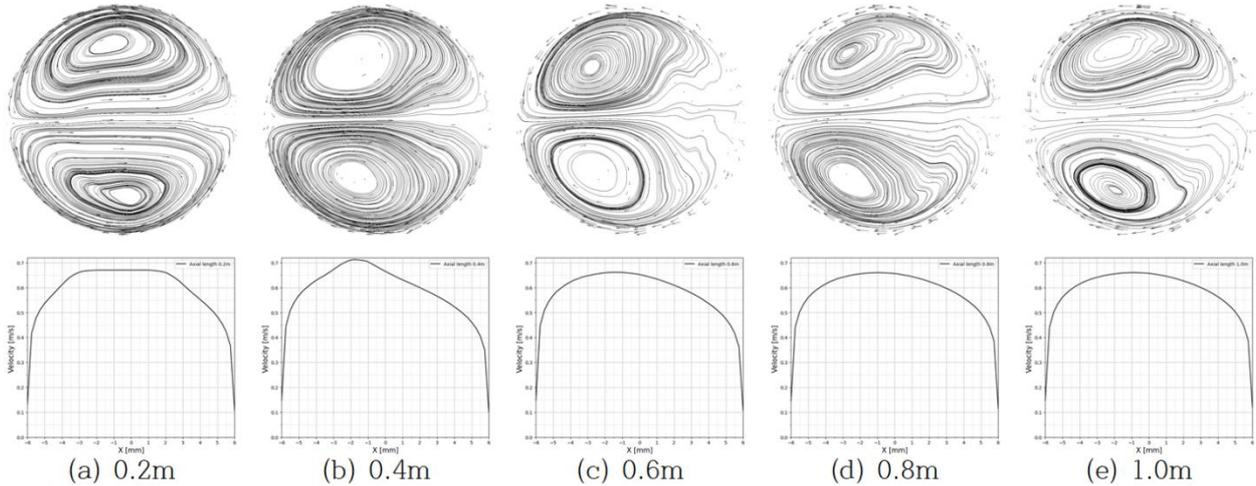
**Figure 3. Development of velocity profiles and secondary flow structures along the axial direction in the first layer ( $Re \approx 50,000$ ).**
