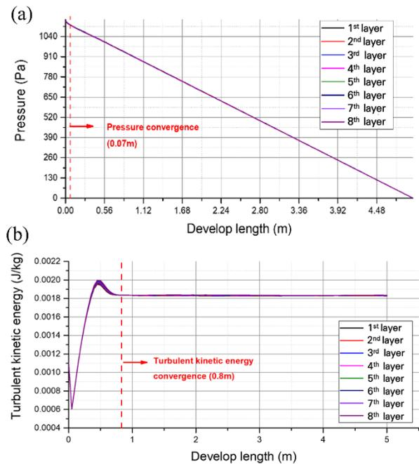
**Figure 2. (a) Pressure development length and (b) turbulent kinetic energy development length for each layer of the helical coil.**
