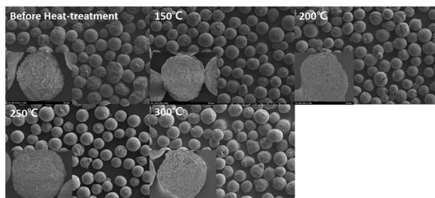
Fig. 1. Scanning Electron Microscope (SEM) Images of Silver-coated Alumina
