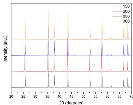
Fig. 3. X-ray diffraction (XRD) Spectra of Silver-coated alumina at Different Thermal treatment Temperature
