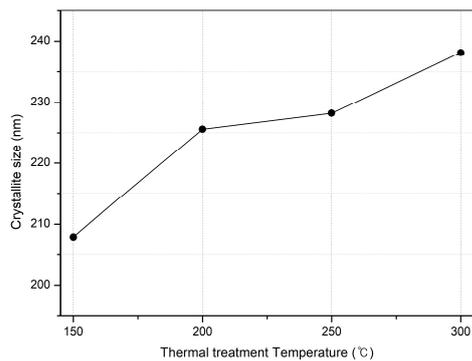
Fig. 4. Average Crystallite Size of  $\text{Ag}_2\text{O}$  of Silver-coated alumina at Different Thermal treatment Temperature
