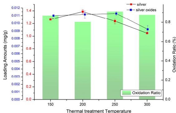
Fig. 2. Effect of Thermal Treatment Temperature on Silver Loading
