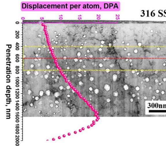
▲ TEM image of void swelling in commercial austenitic stainless steel after heavy ion irradiation (316 SS) [1]
