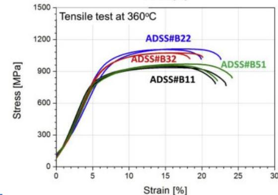
▲ Tensile test results for various ADSS alloys [1]
