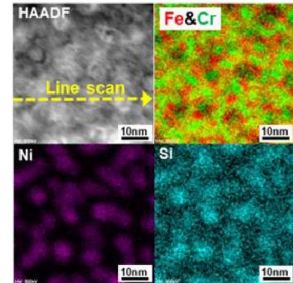
▲ TEM image and corresponding EDS mapping data for showing the presence of spinodal decomposition in  $\delta$ -ferrite after proton irradiation [2]
