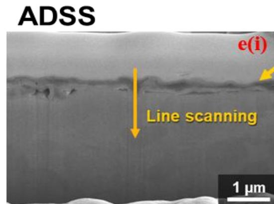
▲ Cross-sectional SEM image of ADSS after corrosion test
