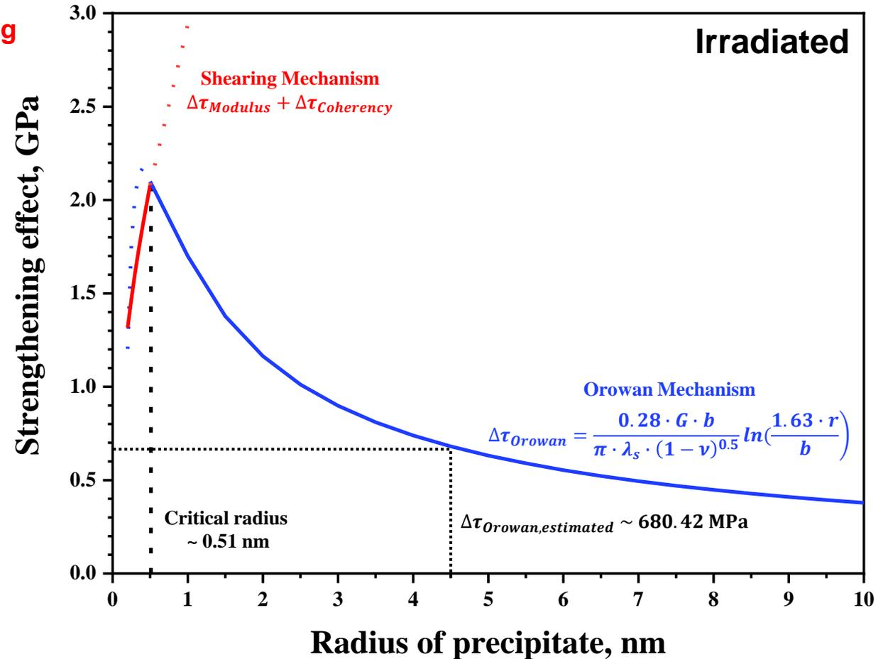
▲ Estimated strengthening effect of  $\gamma'$ -Ni<sub>3</sub>Al precipitates as a function of precipitate radius (nm)
