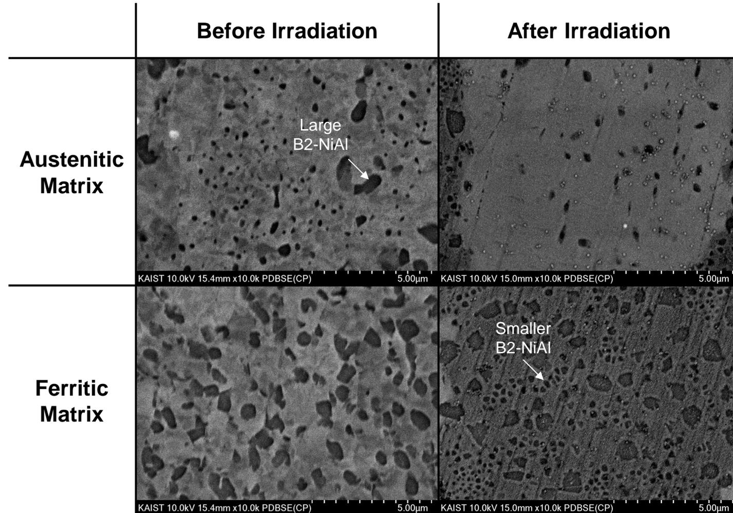
▲ SEM micrographs of microstructural evolution of both austenitic and ferritic matrix in ADSS alloy along the proton irradiation
