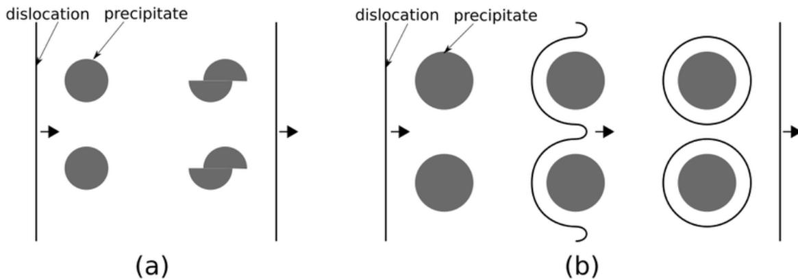
▲ Graphical schematic for precipitate shearing mechanism and bypass mechanism [1]
