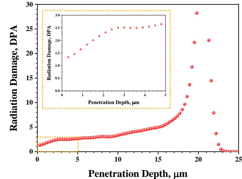
▲ The radiation damage (DPA) as a function of penetration depth ( $\mu\text{m}$ ) in SRIM code simulation
