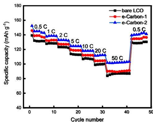
Fig. 3 Rate capability performance of cathodes fabricated with 2 MeV electron beam-irradiated conductive additives at different doses.
