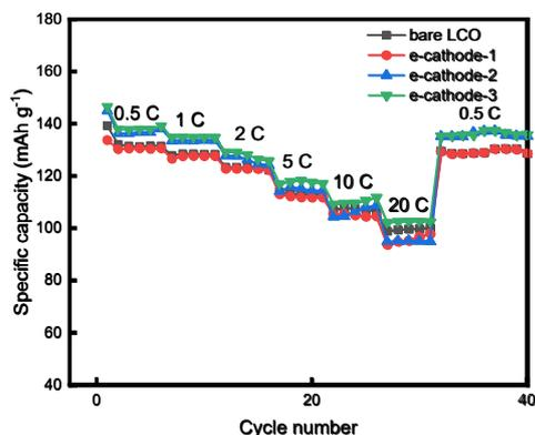
Fig. 1 Rate capability performance of LCO-based cathodes irradiated with 50 keV electron beam at different doses.
