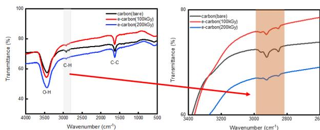
Fig. 4 FT-IR spectrum of conductive additives irradiated with 2 MeV electron beam.
