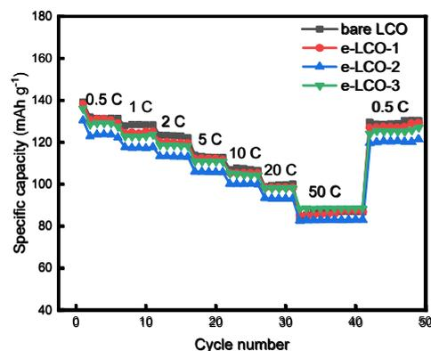
Fig. 2 Rate capability performance of cathodes fabricated with 2 MeV electron beam-irradiated LCO at different doses.
