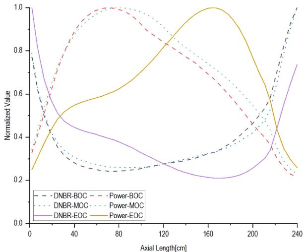
Figure 4. CTF results on the DNBR according to power
