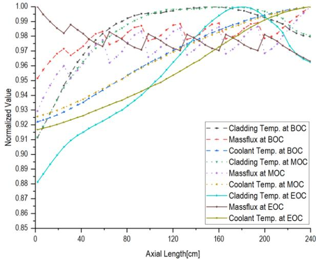
Figure 3. CTF results on the subchannel properties
