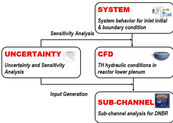
Figure 1. Code system for DNBR [1]
