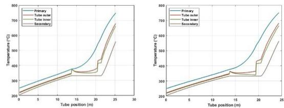
Figure 4: Temperature variation using (a) Zhao and (b) Guo's correlation along the tube length
