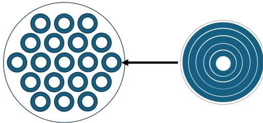
Figure 1: Cross-section of HTR-PM steam generator's shell side and tube side
