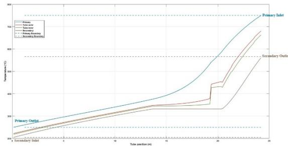
Figure 3: Temperature variation of primary coolant, tube wall, and secondary coolant along the tube length
