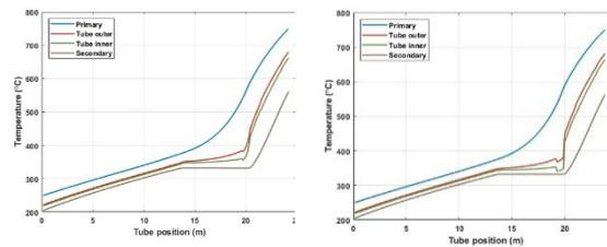
Figure 5: Temperatures at varying tube positions using (a) Xiao and (b) Guo's correlation
