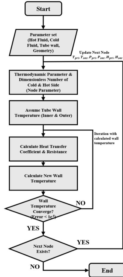
Figure 2: Logic flow chart of computational model
