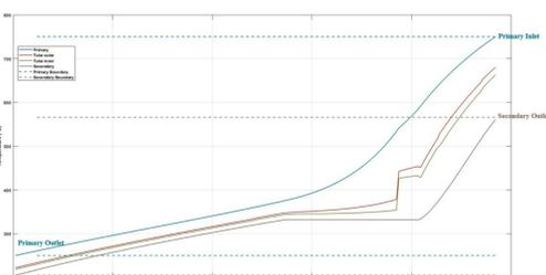
▲ Temperature Variation of Primary Coolant, Inner & Outer Tube wall, and Secondary Coolant along the tube length
