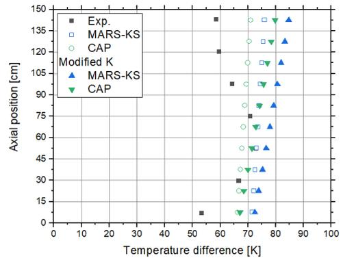
Fig. 8. Comparison of temperature difference at a gap size 40 cm and a heat flux 400W/m<sup>2</sup>
