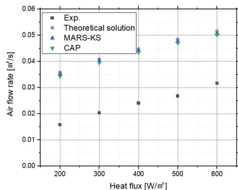
Fig. 4. Comparison of air flow rate with various heat flux.
