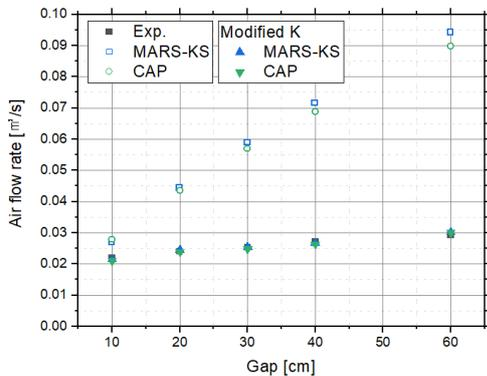
Fig. 5. Comparison of air flow rate with various gap using the modified K.
