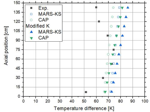
Fig. 7. Comparison of temperature difference at a gap size 20 cm and a heat flux 400W/m<sup>2</sup>
