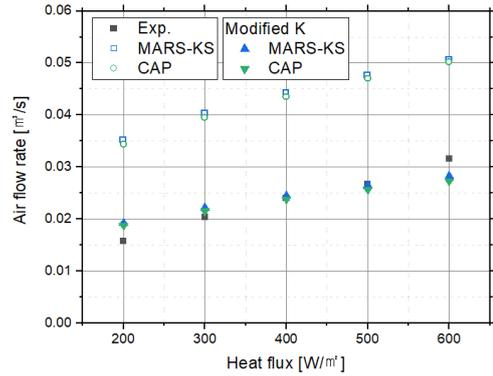
Fig. 6. Comparison of air flow rate with various heat flux using the modified K.
