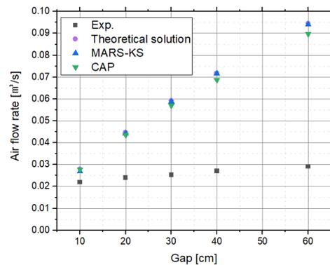
Fig. 3. Comparison of air flow rate with various gap.
