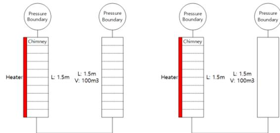
Fig. 2. Nodalization of MARS-KS(Left) and CAP(Right).
