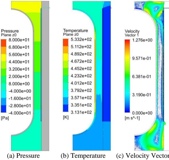
Fig. 4. Simulation results for Case 2 ( $\epsilon_{\text{Pipes}} = 0.68$ ).
