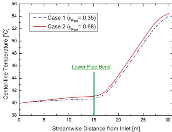
Fig. 7. Center-line water temperature profile along the streamwise distance from the inlet.
