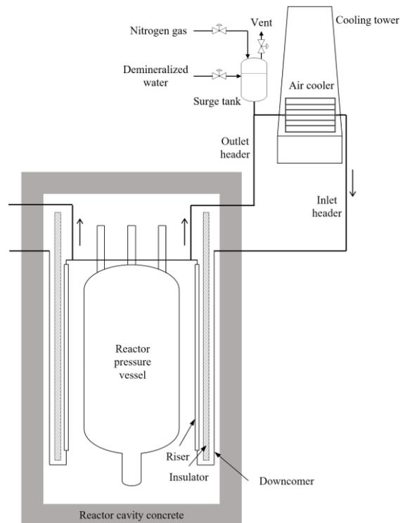
Fig. 1. Conceptual diagram of the HECTAR RCCS.
