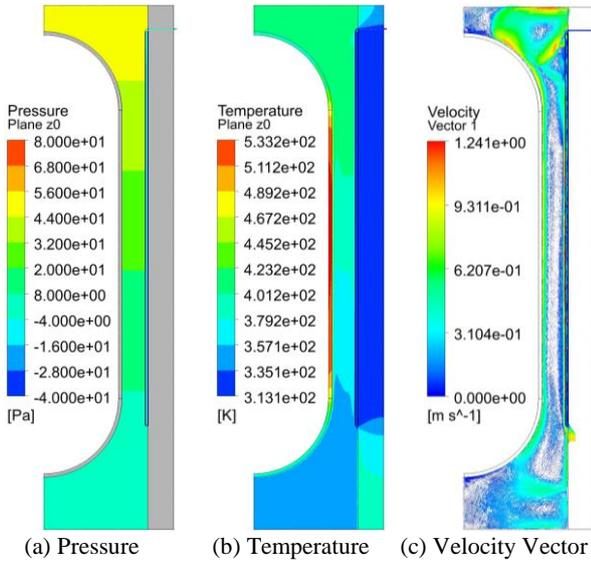
Fig. 3. Simulation results for Case 1 ( $\epsilon_{\text{Pipes}} = 0.35$ ).
