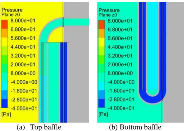
Fig. 5. Pressure distributions over the top and bottom baffle interface areas between the atmospheric and the insulating air (Case 2).
