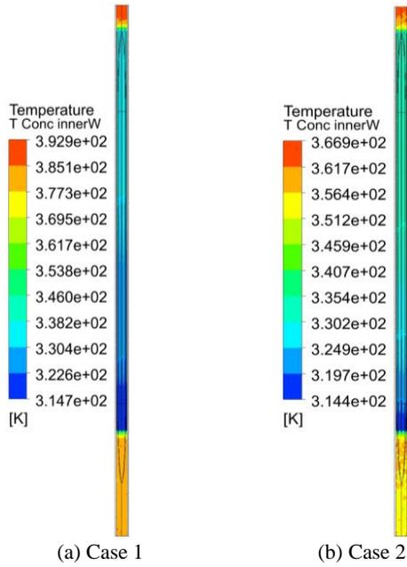
Fig. 6. Temperature distributions on the inner surfaces of the bare concrete and the pipes and connecting steel plates (view from the center)
