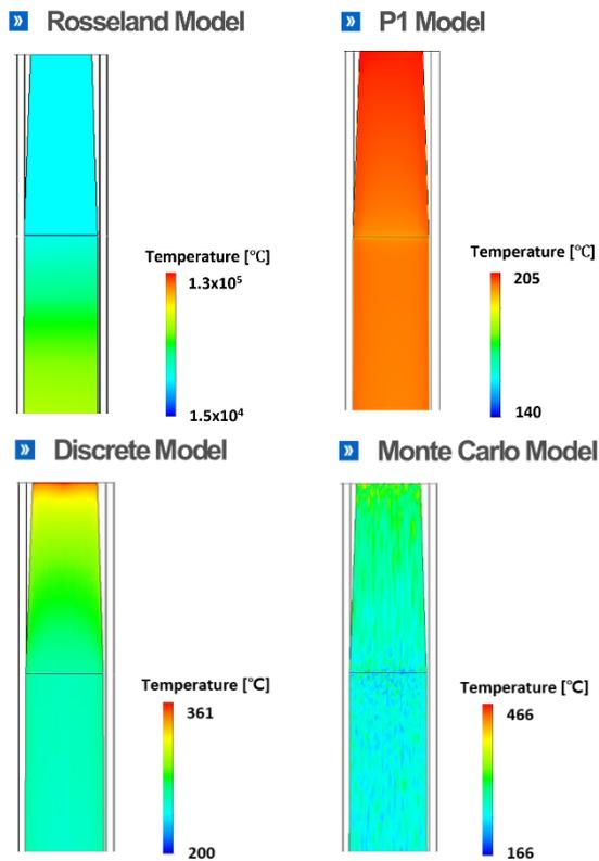
Fig. 3 Temperature distribution by radiation model in RPV
