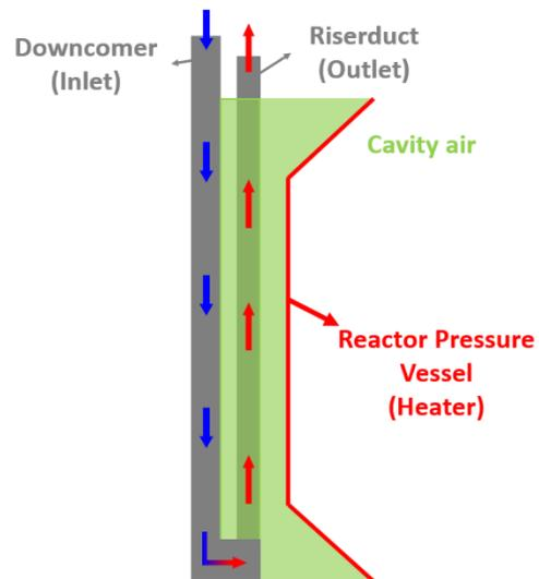
Fig. 1 Schematic of MHTGR RCCS system
